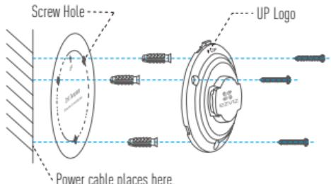
4. Fix the base cover on the base (OPEN right on the UP).
